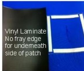
6. Tape and turn the the edges with the high tack adhesive.
