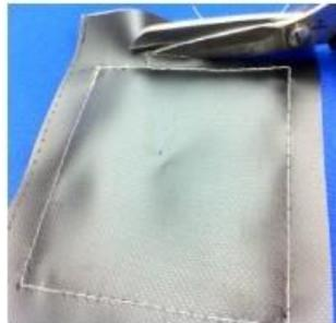
Another way you can handle smaller tear repairs is with a product called tearaid®. Tear-aid® is flexible cut to size patch with a single sided aggressive adhesive that will stick to a variety of fabrics. The patches come in **Type A** for all fabrics including Sunbrella® and **Type B** for vinyls . You just clean the fabric according to their instructions and stick the patch on both sides of the fabric, rub and your done. The patch is opaque in color, so it blends pretty well.
